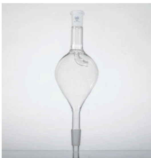
Straight, with standard ground cone and socket.
